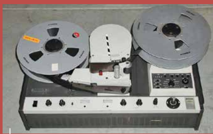
The Ampex 660 was an early broadcast-quality video recorder. Jim Songer bought one of the first examples but modified it extensively for work in the video assist system.
